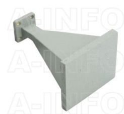
LB-28-20-ASPO Standard Gain Horn Antenna 26.5-40GHz 20dB Gain Rectangular Waveguide Interface
